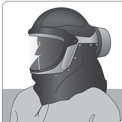
(C) Powered, air-purifying, ventilated helmet respirator.
