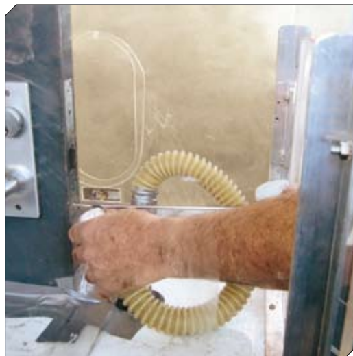
Figure 3: Side view showing the operator using the vacuum hose to 'shadow vac' below the screw as it is unscrewed from the lock housing.
