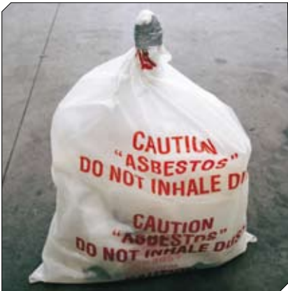
Figure 8: An asbestos waste bag with appropriate warnings.
