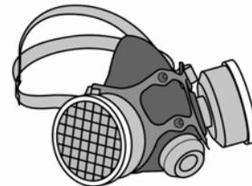
(B) Half-face, particulate filter (cartridge) respirator
