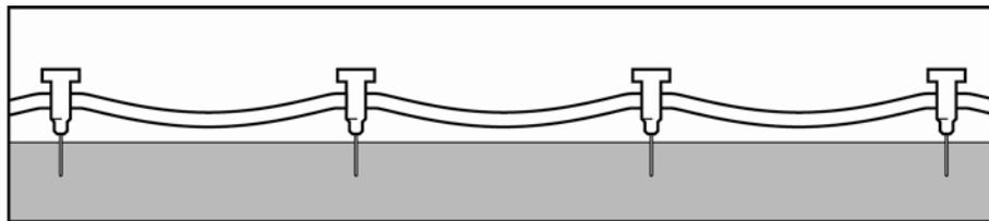
The asbestos is soaked by the introduction of water or other wetting agents through an appropriate applicator that consists of an injection head with numerous side holes or outlets through which the water or wetting agent is fed to the asbestos.
